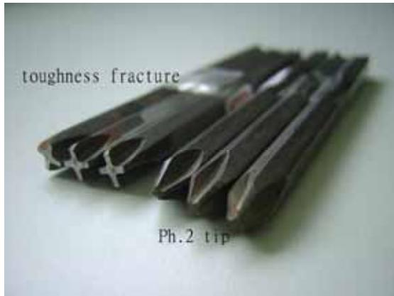
**Fig. 3.** Profiles of Ph.2 tip of screwdriver bits before and after torsion testing.
